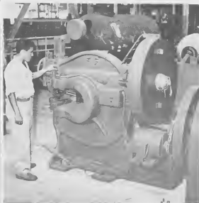
TWO STAMPING machines represent the old and the new in Lago's shops. The new machine, above, is capable of generating 156 tons of force which is just enough to punch out a two-inch diameter hole in a one inch metal plate. Pictured with the new machine, which also shears, notches and copes, is C. Lae. Below is A. Boezen.
